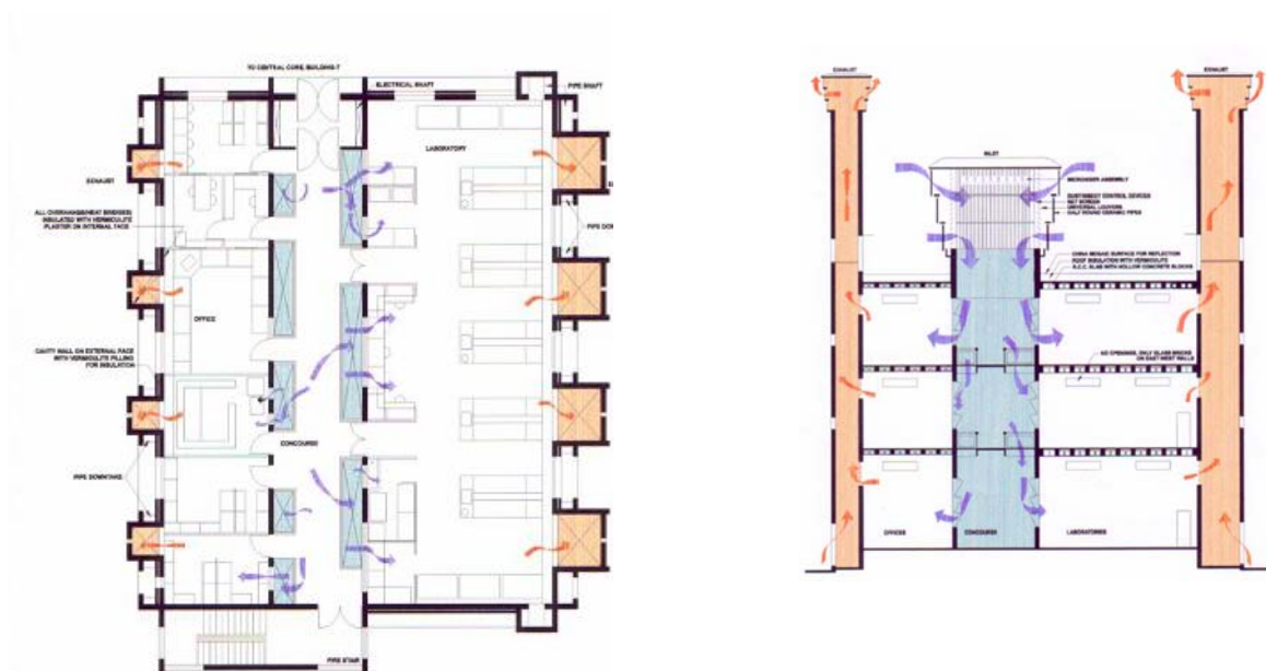
Figure 1 Plan and section of a PDEC Building
